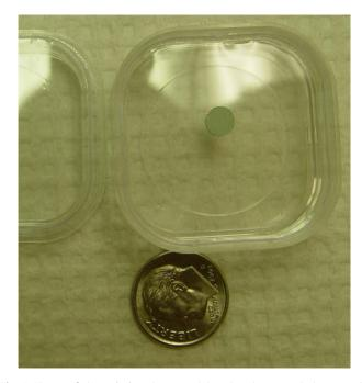
Fig. 1. Picture of sintered plutonium containing zirconia-magnesia inert matrix fuel ( $Zr_{0.76}Mg_{0.10}Pu_{0.078}Er_{0.062}O_{1.9}$ ).
